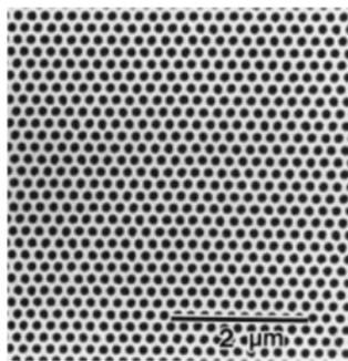
Nanoporous anodized alumina
