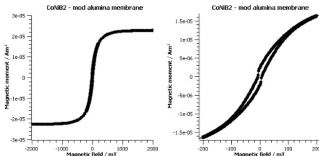
Magnetometry (VSM) on tube array (in template), field  $\perp$  to tube axes
