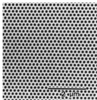
Nanoporous anodized alumina
