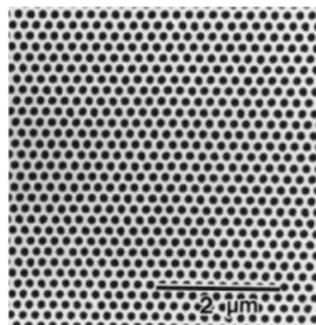
Nanoporous anodized alumina
